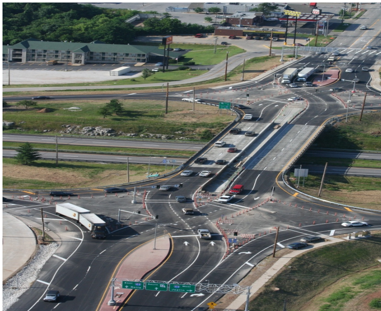
Figure 6- Diverging Diamond Interchange Design (MoDOT 2016)
